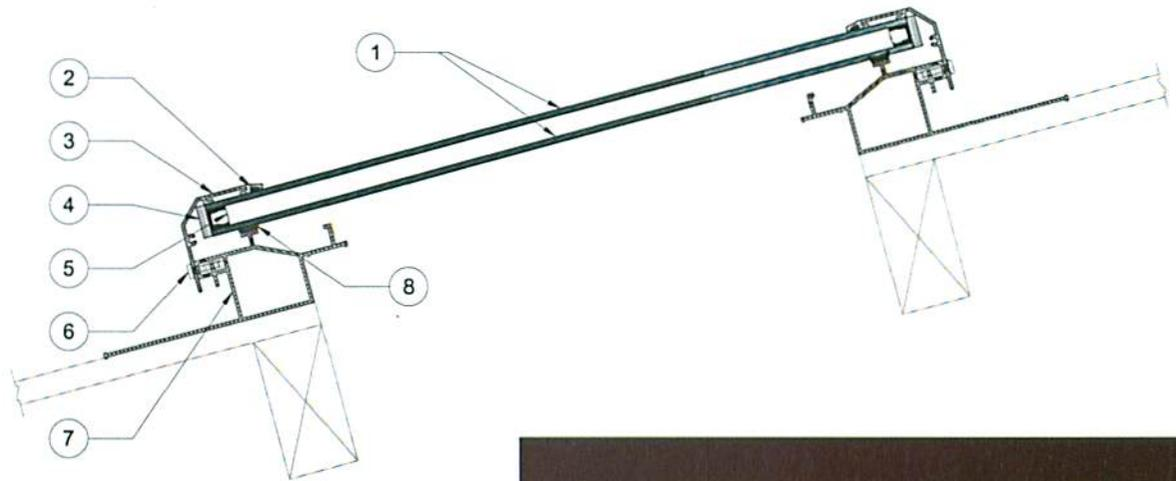
**MODEL G-PVCSR (SELF FLASHING FIXED - GLASS GLAZING)**
