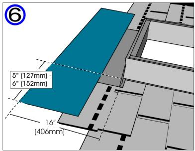
Replace remaining shingles. Apply weatherstripping to top of curb. Tack weatherstripping with roofing nails. Mount and secure skylight with screws as shown
