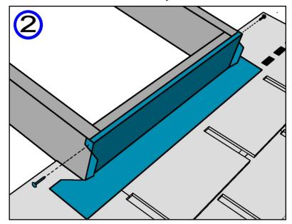
Install step flashing and shingles beginning at the bottom as shown (3a).
