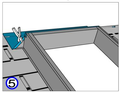
Overlap head flashing with underlayment as shown
