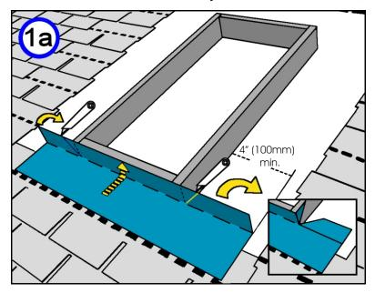
Next, Install Underlayment against two sides of curb (1b). Again start at top of curb, work underlayment tight into corner, and finally out on roof deck. Trim corners as shown. Cut corners and fold as shown.
