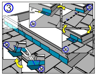
Install side counter flashing, ensuring bottom tabs overlap tabs of sill flashing. Nail into top of curb. Squeeze tabs with pliers to lock corners.
