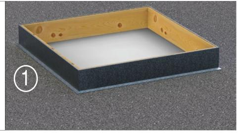
Dry fit skylight to curb to ensure proper fit.
