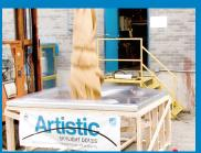
testing to evaluate the FPS skylights' structural strength & integrity. Final results showed that the skylights met & exceeded OSHA's guidelines for skylight fall protection<sup>1</sup>. With the help from Exova
