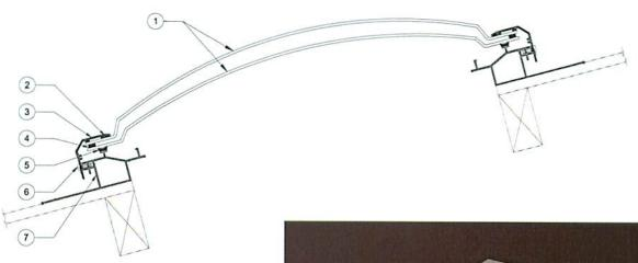
MODEL PVCSR (SELF FLASHING FIXED - ACRYLIC DOME GLAZING)
